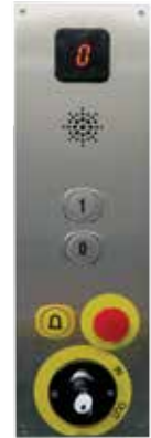
Lock switch IN – OUT to disable commands and light curtains (exclusive use for goods only transport)
